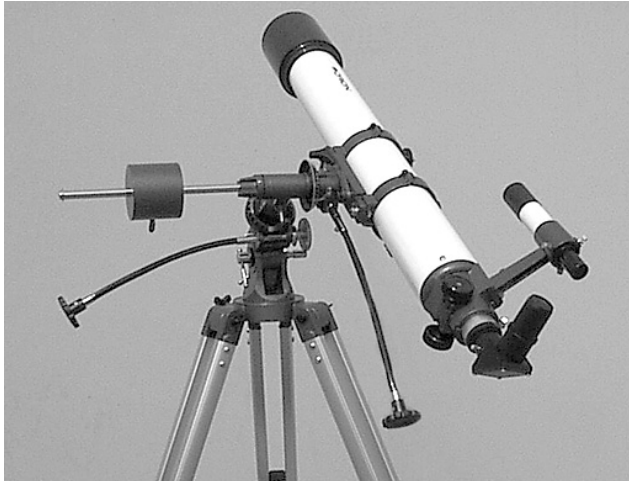
Figure 6a. Telescope pointing south. Note that in all these illustrations, the mount and tripod remain stationary; only the R.A. and Dec. axes are moved.
