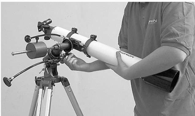
Figure 3c. Preparing the telescope to be balanced on the Dec. axis by first releasing the Dec. lock knob.
