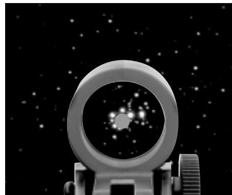
Figure 7 EZ Finder II superimposes a tiny red dot on the sky, showing right where the telescope is pointed.
